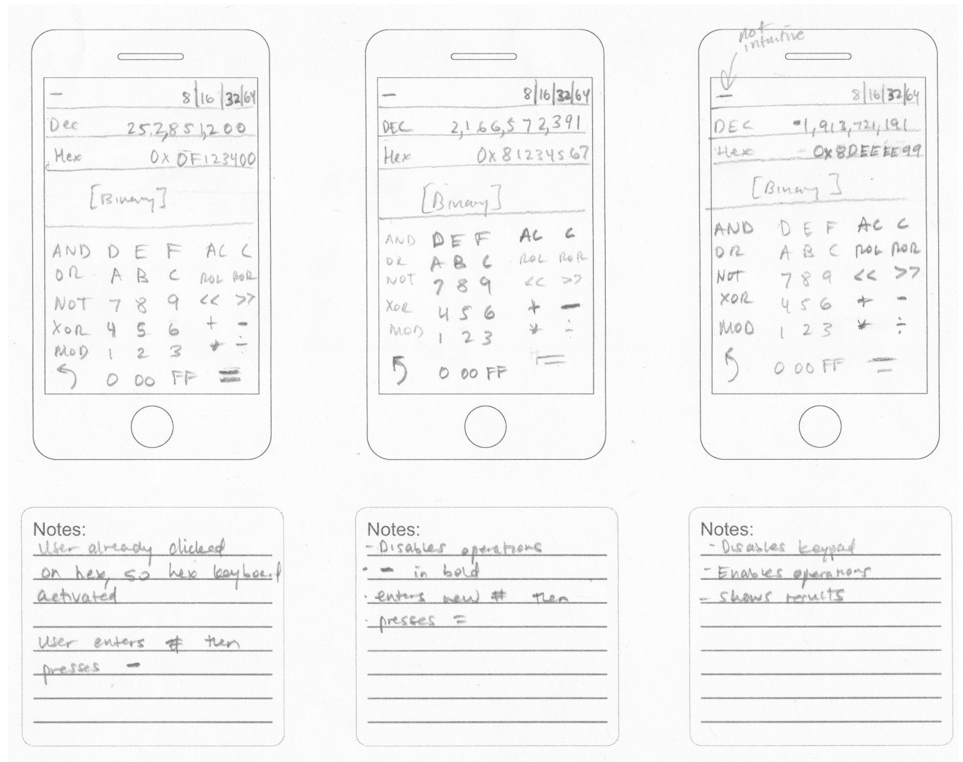
Figure 6: A storyboard for subtracting a larger hexadecimal number from a smaller one (as in the first scenario).
